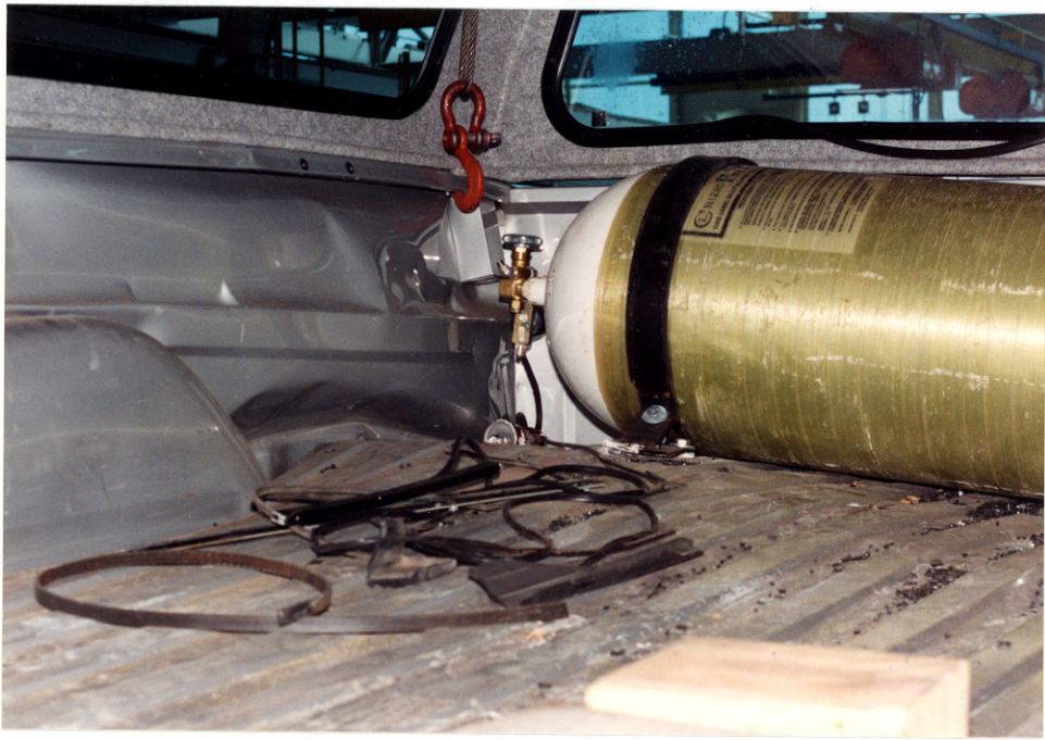
13. Angular view of the add-on tank from the right side showing deformation resulting from the CNG tank failure
